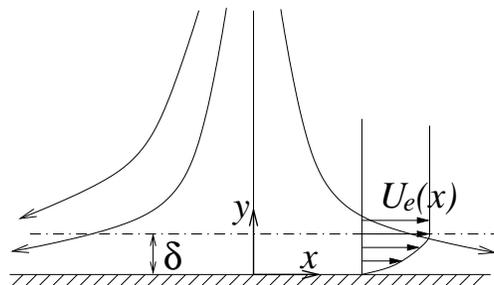
**Problem 3:** Consider a semi-infinite porous plate aligned with a free stream of uniform velocity  $U_\infty$ . A constant suction velocity  $v_w = -v_o$  exists on the plate surface, so that far from the leading edge the boundary layer approaches a solution independent of  $x$ , as shown in the figure below.
